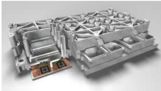
Fig. 3: SKiM, the first ever 100% solder-free IGBT module Basic design of the IGBT module: sintered chips, no base plate, pressure contacted via springs.
